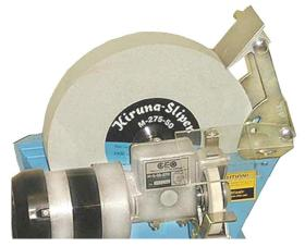
After adjusting the desired grinding angle, screw firmly the three screws to ensure the stability of the grinding –support. Following is instructions about how to grind different tools.
