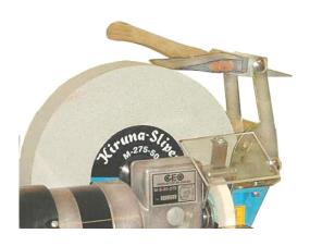
If you are grinding tools with a big angle turn application nr 1. For example different types of scissors. Just remember to properly draw the screws
