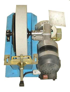
An out-flow is available to adjust the grind stone of the Kiruna-grinder. Start your adjusting from the edge to the center to avoid splintery.
