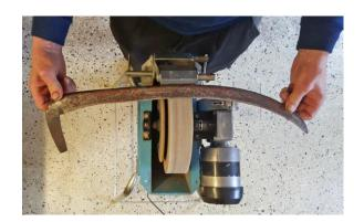
If the stone has become oval. You can easily restore it with a paint scraper. The steel should preferably be made of hard metal. Sure that the stone is dry before beginning.
