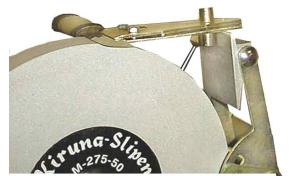
Place the grind jig on the grind stone according to the illustration. Grind one side, then turn both the knife and the grind-jig a half turn and continue grinding.
