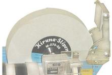
Grind jig for chisel, plane-iron, black-steel etc. This grinding is a good assistance facility to all, It goes very rapidly to grind and if you desire to examine the tool while grinding you do so and continue later on. Keep in mind that the tool can be placed in the same position. This allows you to avoid damages under the grinding stage. This can as well be used with different types of tools.
