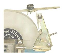
To start with grind the plane-steel straight. When you are ready turn it slightly to each side to ensure you a small contrast of edges and a good result.
