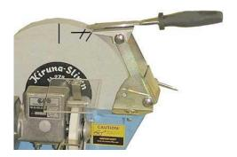
There are 3 screws on the grind stone that you can adjust as you wish. To obtain a bigger area turn the lower long screw so that the wing-screw falls on the side beside the grind plate.
