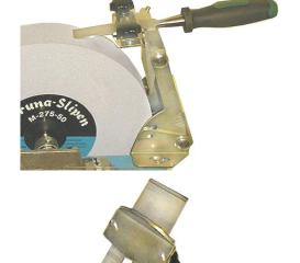
This is how you assemble the jig on a plane-iron. As you can see I have turned the jig a whole round with comparison to the chisel. Just remember to round the plane-steel while grinding. This minimize the possibility of stripes that can otherwise be formed by sharp edges of plane-steel.
